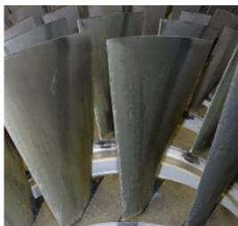
16,000 hrs with AAF's EPA E12 filtration and no water washes
