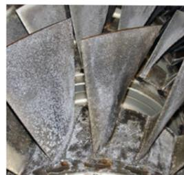
8,000 hrs with high velocity bag filters and frequent offline water washes
