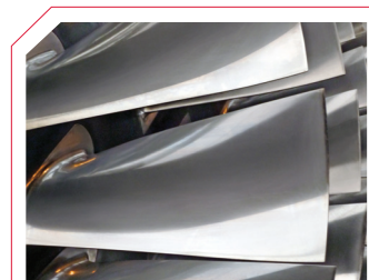
Figure 3: GT compressor blade with AAF HEPA (8,000 hours)
