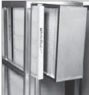
2" PerfectPleat® pleated filters are shown installed in the prefilter track on the upstream end of the housing in front of AstroCel® HXC final filters.
