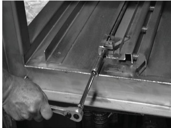
2. To prevent filter gasket from sticking to the housing sealing surface after being compressed for an extended period, the entire face of each new filter gasket may be coated with an optional silicone grease before being installed. A 1/8" - 3/16" diameter bead of this silicone grease can be applied to the middle of the entire 3/4" wide filter gasket.
