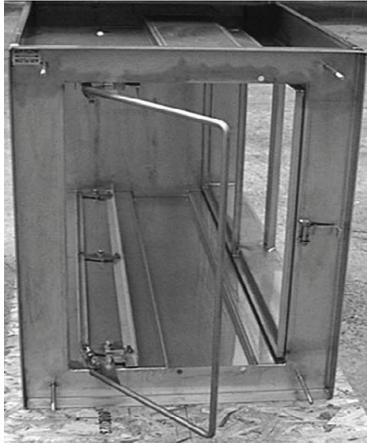
2. To install the filter (or adsorber) in the housing, orient the filter so that the T-clips on the filter overlap the mechanism and the gel seal channel is aligned with the knife edge of the housing.
