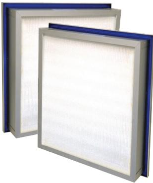
Filters for ceiling grid systems incorporate an integral ¾", 1", or 1¾" filter skirt on the downstream perimeter. The filter media is formulated from all-glass microfiber with a water-repellent binder. The glass microfiber contains less than 10 PPM of boron when digested in acid and analyzed via Inductively Coupled Plasma Atomic Emission Spectroscopy (ICP-AES).
