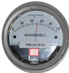
*MEGAPleat® M8 filters in service over eight months show a resistance of only 0.51" w.g. Standard capacity filters would have been changed out three times at this point.*
