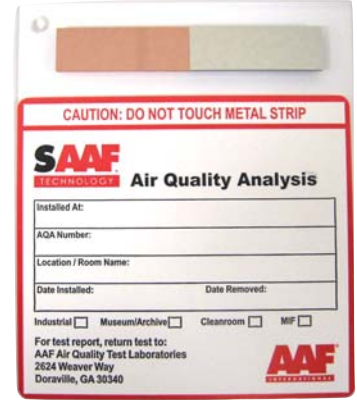
Reactivity Monitoring Coupon — Glass p/n: 392-801-000
