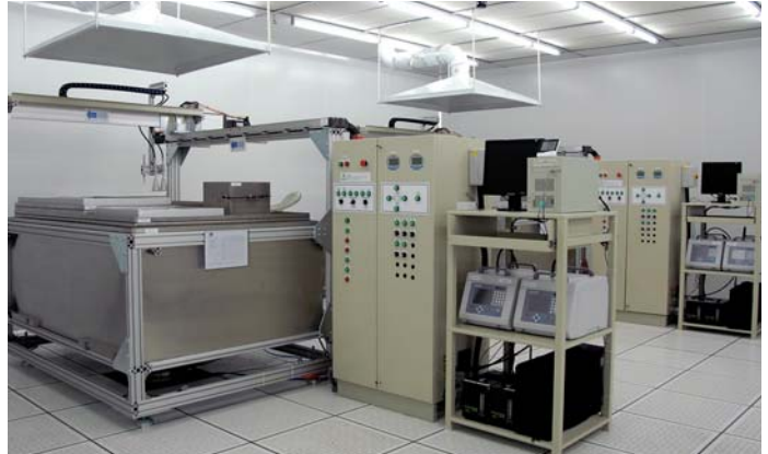
AAF's testing procedures for overall efficiency include laser particle counters with liquid or solid aerosol challenge. Pinhole leaks can be detected using either AAF's proprietary static scan test or automatic scan testing.
