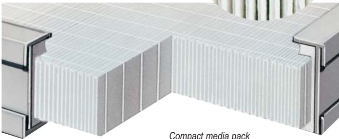
Compact media pack available in sizes from 2" to 4" deep.
