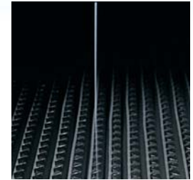
Scan test showing leak indicated by a smoke trail.
