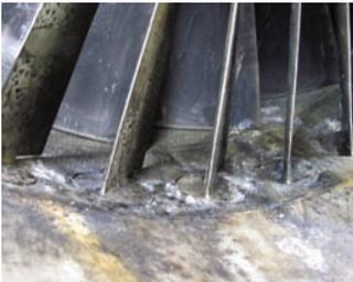
Combustion air intake blades showing saline contamination
